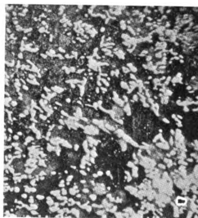
Microphotographs showing the varied nature which can be possessed by practically similar compositions of bronze
